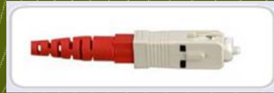
Subscriber connector (SC) multimode
